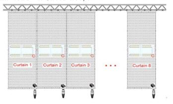
The PC controller has 4 boards built inside. Each board has two data outputs. The PC controller is a slave to the V- controller/main controller. As mention above, one group of data output can control maximum 3412 led pixels. One led curtain has 2,400 leds, so one data outputs can connect to one led curtain only. So you need to select "A line with a slave".
