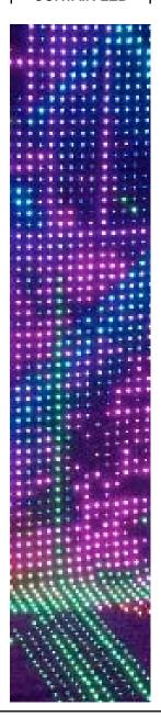
There are 24x100 = 2400 leds in the curtain, you need to set up Width: 192 and Height: 100. Since you are going to directly control the led curtain with computer, select "Network Adapter. Click OK.
