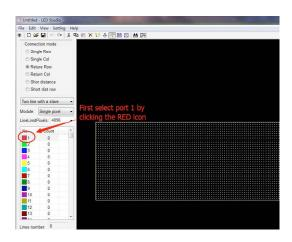
Now move your mouse to the no. 24 led from the left side at the bottom line. This is the first led in the first led curtain. The value below tells you if you move to the correct column.
