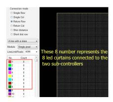
Now select number 1 first by clicking it with your mouse. Then in the right side of the window, select the FIRST led in the led curtain by right clicking your mouse, hold the mouse and move to the last led in the curtain, so that to cover the whole led pixels in the first curtain. You can see if you have covered 24x100 leds by checking the figures at the bottom.
