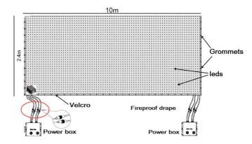
The power box has an extra clamp. Fix the clamp to the power box, the box can also be mounted to truss if needed.
