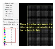
The 8 number represent the 8 led curtains connected to the 2 sub-controllers.
