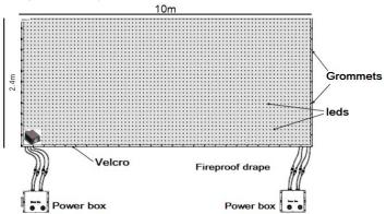
DesignCurtain Pro has grommets and holes at its four sides, users can fix the drape to truss or other structures easily and quickly.
