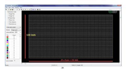
The "Connection mode" means how the leds are connected on the curtain. As mentioned before, leds are embedded in the curtain like this, leds are turned by row.
